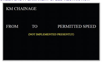
This function is futuristic and not implemented presently. For full fledged implementation, railways have to device a mechanism to feed the en-route permanent speed restrictions into the driver display. It would also require logistics for transferring the speed restrictions en-route from a base station to a moving train.
