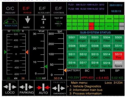
In the sub-system status menu, the names of the sub-systems are listed. To navigate to default screen, press <HOME>. To navigate to list of screens, press <ESC>. The isolated sub-system will be shown in red.
