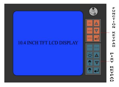
The Driver Display has two sets of keypads positioned in different clusters. One set is known as "PIXY" display control key pad & another is known as "Function" keypad. The PIXY control keypad has 8 keys and provides exactly the same control as being done in the old type of 4x40 text display. The "Function" keypad has 6 keys, each assigned to a separate function.
