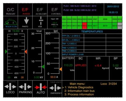
The temperature screen provides various temperatures recorded by sensors and the same can be compared with the converter input power. The temperatures of transformer oil, traction converter oil and traction motors are displayed alongwith converter input power for each bogie
