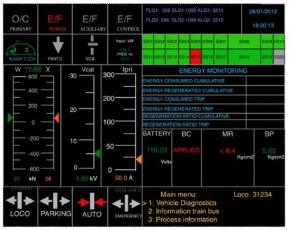
The screen for energy monitoring displays the energy consumed and regenerated. The cumulative value is the one taken from the NVRAM of DIA computer, which is available on MVB. The trip energy is calculated by the driver display itself from the time of switching ON. This value is not saved in any memory and will vanish once the locomotive is OFF. Trip energy can be used for comparison of driver performance under identical conditions of operation.
