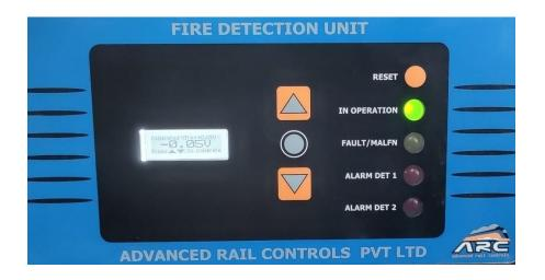
To calibrate press either Up/Down button now another screen appears "To calibrate press ( $\bigcirc$ ) button". Then it shows "Calibrating......". When calibration is completed, final screen appears "Calibrated voltage = +/-0.05V".
