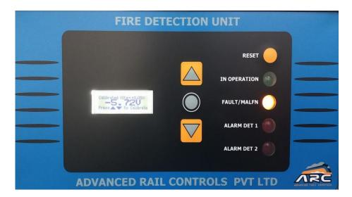
If any smoke is detected at any suction point of the pipe either Alarm smoke detector 1 or Alarm smoke detector 2 (Red) will glow.
