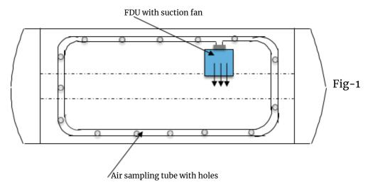
The condition of the sampled air is continuously monitored using an air monitoring system. A sample of the air is passed through an air filter and the flow is monitored. In case the air contains dust particles beyond the acceptable levels, it could affect the performance of the FDU and also may lead to false alarm. If the dust content is more than acceptable, the air flow measuring system will generate alarm to enable cleaning of the FDU.
