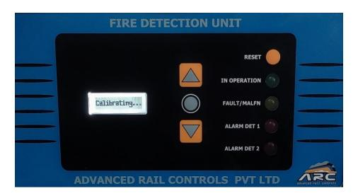
Connect the suction pipe to the FDU. When all the holes of the pipe are closed Fault/Malfunction LED (Yellow) will glow.
